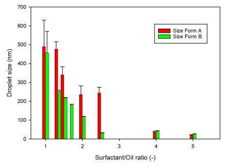
**Figure 2.** Relationship between the surfactant/oil ratio and the droplet size for formulations A, containing Maisine<sup>®</sup> CC, and for formulations B, containing Labrafac<sup>TM</sup> Lipophile WL1349 (n = 3).
