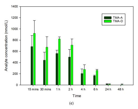
**Figure 7.** Plasma concentration versus time curves of TMA-related metabolites, TMA-A and TMA-D, considering TMA suspended in water (a), solubilized in formulations A.1 (b), and B.1 (c) (n = 3, data are presented as mean  $\pm$  S.D.).
