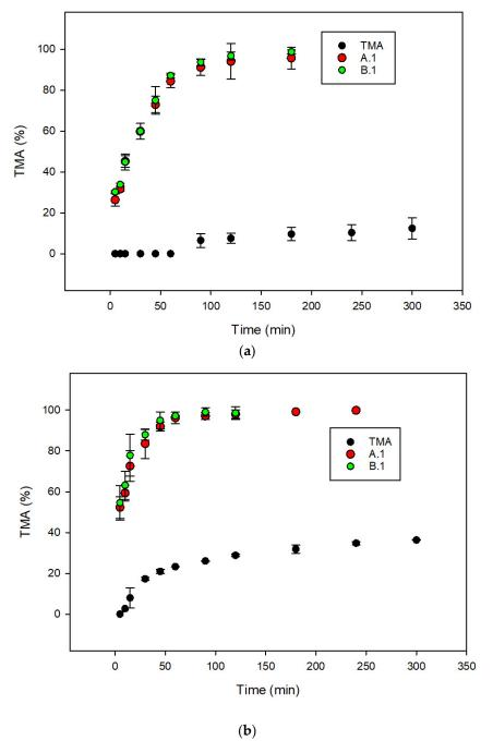
**Figure 3.** Dissolution profiles of TMA and TMA delivered in formulations A.1 and B.1 obtained using FaSSIF (a) and FeSSIF (b) buffers as dissolution media.
